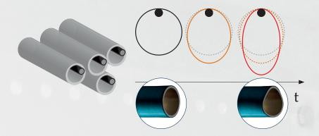
This improper storage produces in short times (dependent on variables such as thickness, diameter, material etc.) a modification of concentricity, generates a permanent damage and the sleeves became unusable. Often also similar solutions are used in an attempt to rationalize space and manage large amounts of sleeves but, de facto and quickly, turn out to be ineffective and inconsistent.
